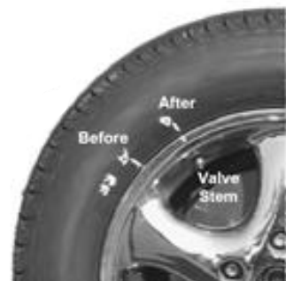
3" slip after mild driving (over)
