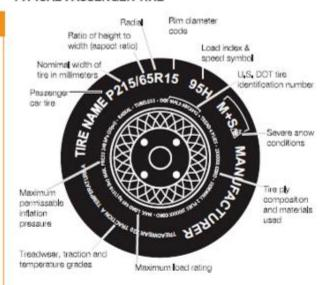
The letters "DOT" certify compliance with all applicable safety standards established by the U.S. Department of Transportation (DOT), Adjacent to this is a tire identification or serial number. This serial number is a code with up to 12 digits that are a combination of numbers and letters. The last characters are numbers identifying the week and year of manufacture. (For example, "1502" means the fifteenth week of the year 2002.)
