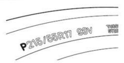
The maximum load capacity stamped on the sidewall of a P-metric tire is reduced by a factor of 1.1 when used on a light truck, a sport utility vehicle, or a trailer.
