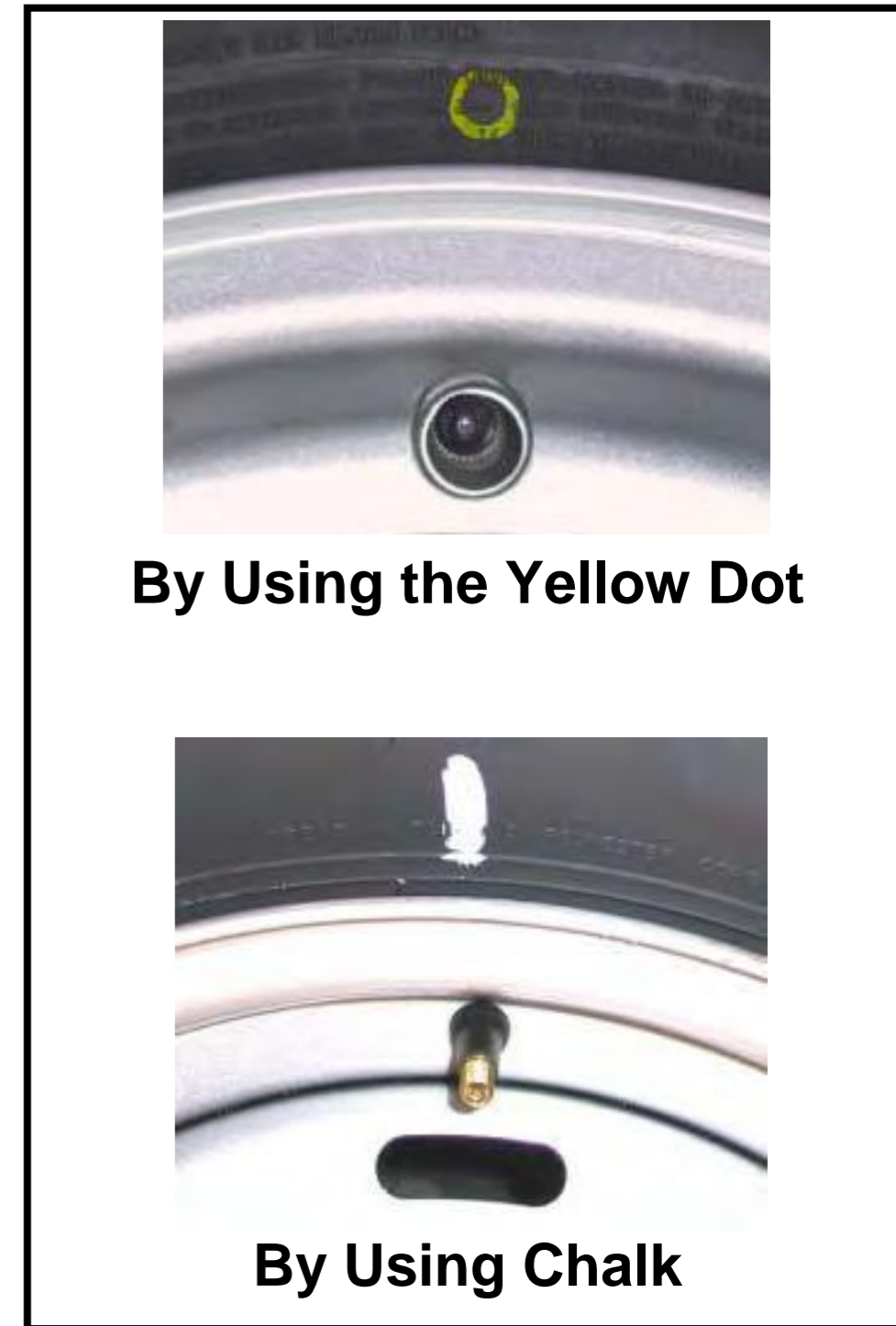
Index the Valve to the Tire
