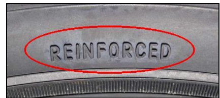
Figure 1. “Reinforced” marking on sidewall.
