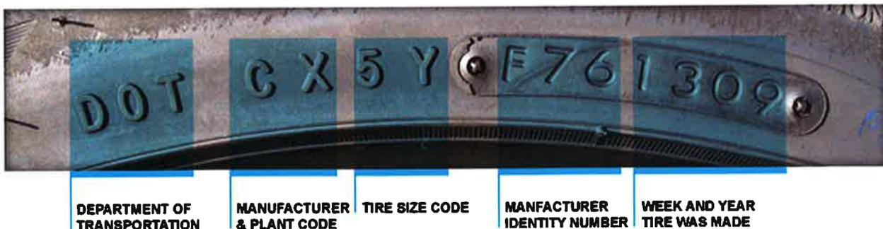
Prior to 2000, the year code of the manufacture date was represented by 1 digit instead of 2 (*i.e.*, 517 would represent the 51st week of 1997). In the absence of the decade triangle, this tire would have been made during the 51st week of 1987.
